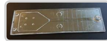
Injection molded chip R2R-imprinted \mu F chip
